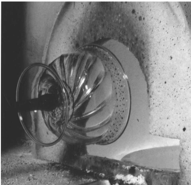
Fig. C. The vessel is then exposed to the heat of the furnace. This softens the rim, melts the enamels, and fuses them and the gold leaf to the glass.
